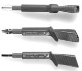
Three self-retaining test probes with touch protection for the connection of measurement cables with 4 mm banana plugs, or with touch protected plugs for sockets with an opening of 3.5 mm to 12 mm, e.g. CEE or Perilex sockets etc.
